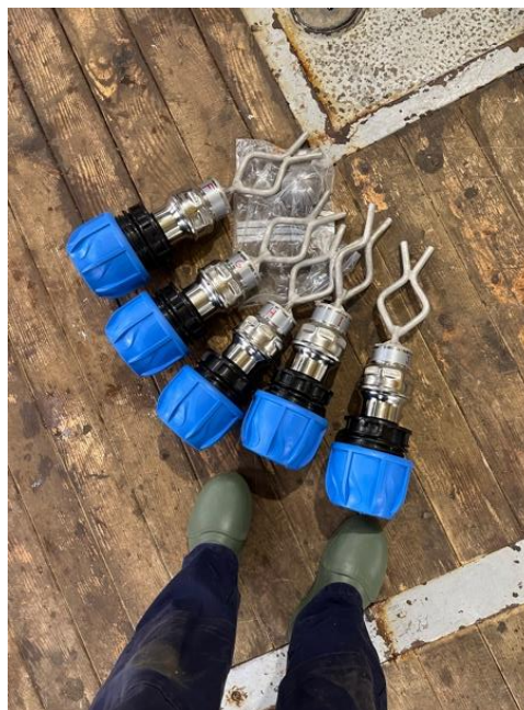
Figure 3. New push core valves with bigger openings
