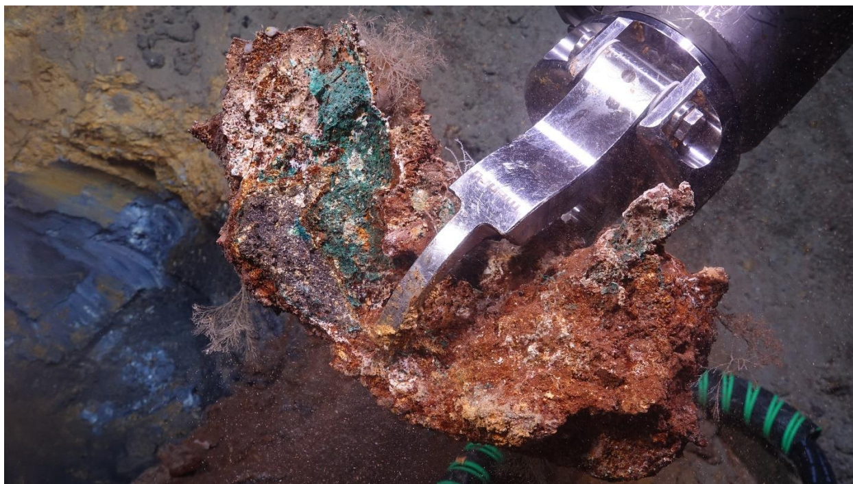
Figure 11. Image showing atacamite precipitation on one of the samples from Grøntua.
