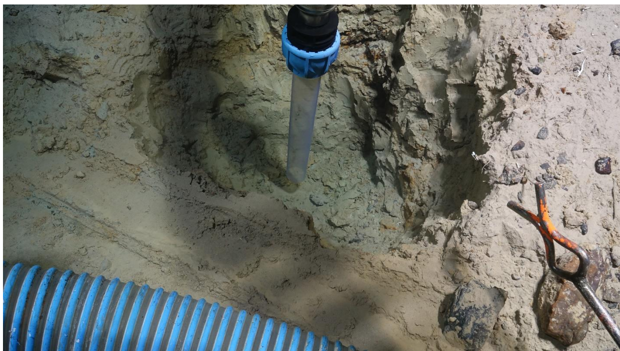
Figure 17. Push core sampling in dredging hole at DeepInsight Hill during ROV21.
