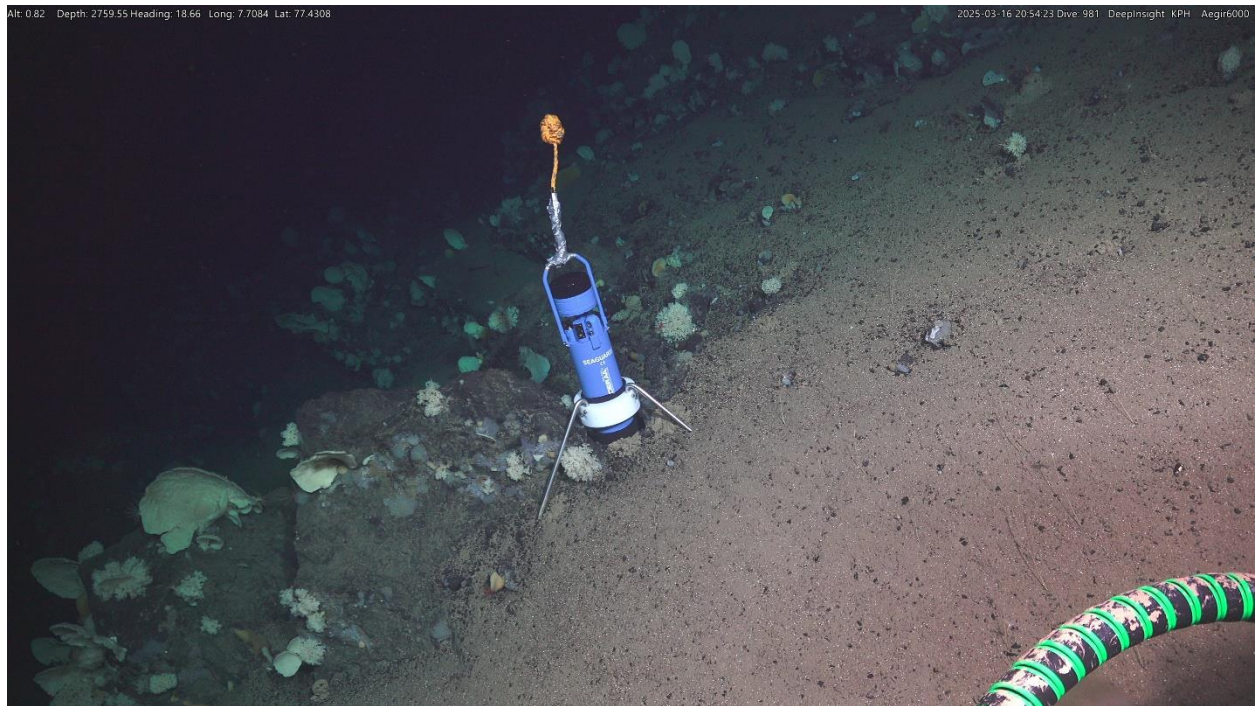
Figure 7. Picture from the first retrieval of the SeaGuard in proximity to the sulfide deposit during ROV08.
