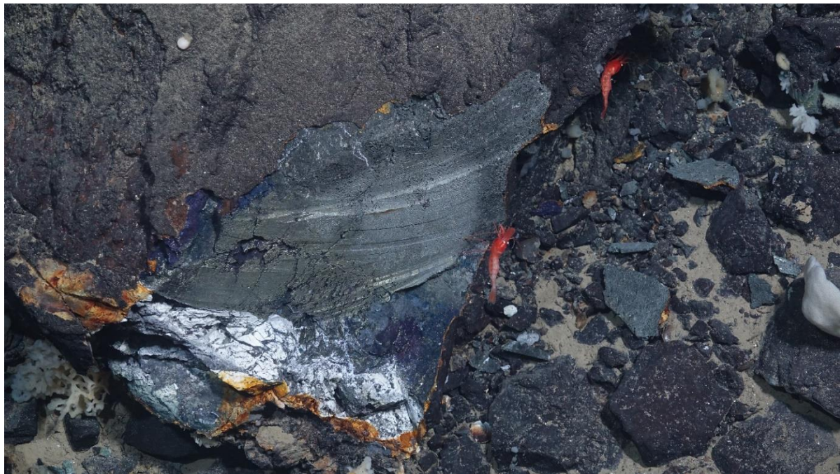
Figure 5. Massive sulfide sawed off using the grinder at the sulfide deposit during ROV06.
